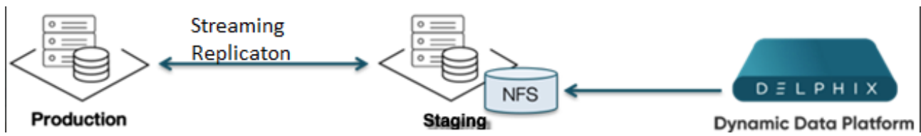
Block Diagram of Linking Architecture Between PostgreSQL Environments and the Delphix Initiated Backup Platform.
