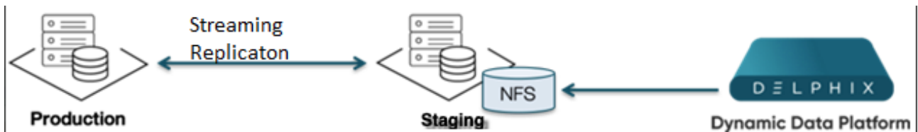
Block Diagram of Linking Architecture Between PostgreSQL Environments and the Delphix Initiated Backup Platform.
