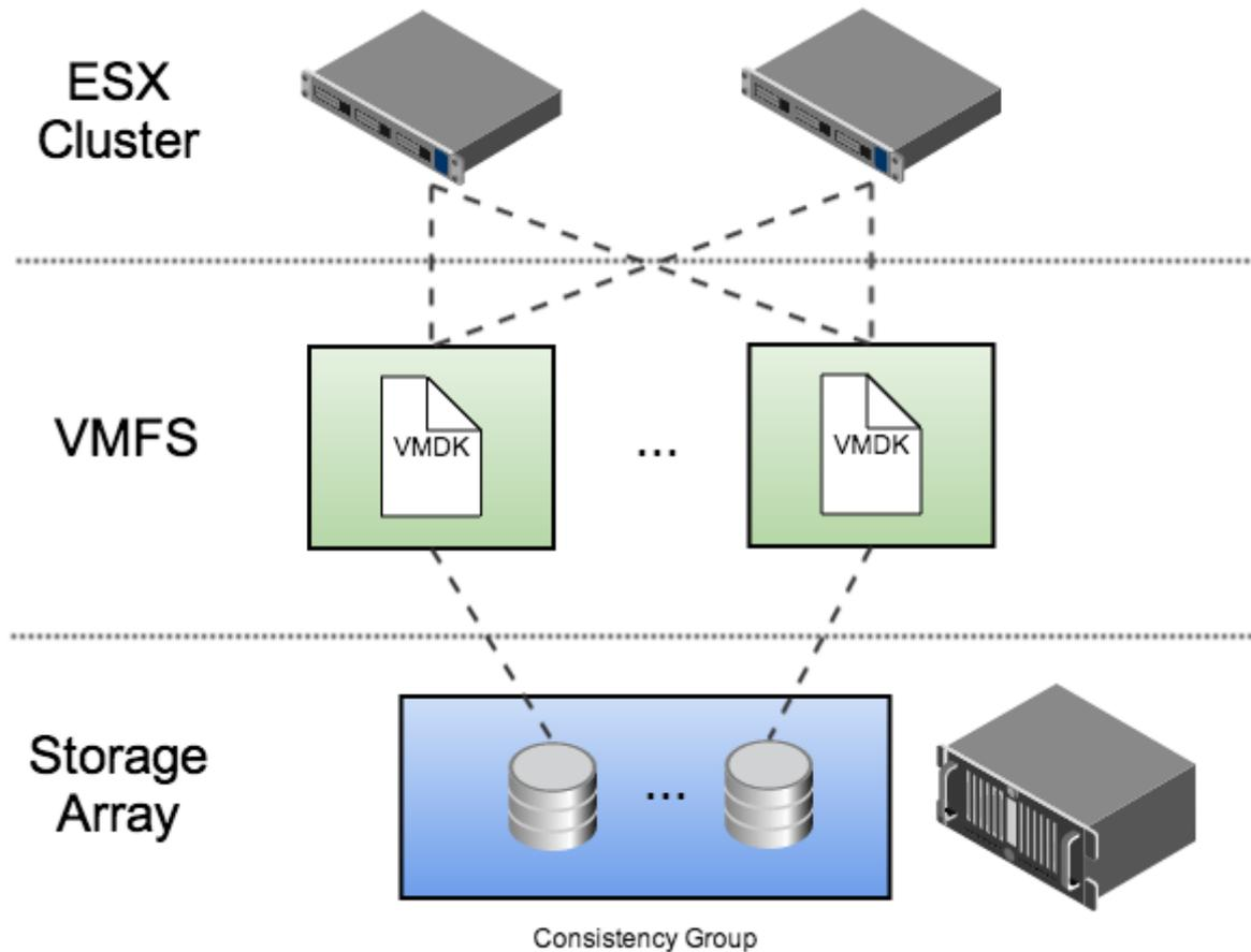
This architecture is designed to isolate I/O traffic to individual LUNs while using the most commonly deployed VMware components. In this example, each VMDK file is placed in a separate VMFS volume. Each volume is exported to every node in the ESX cluster, allowing the Delphix Engine to run on any physical host in the cluster.
