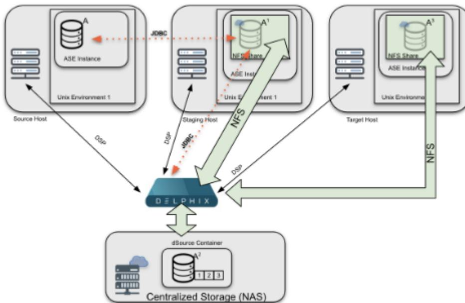
*Architectural diagram of a common Delphix deployment (configurations vary depending on RDBMS platforms)*
