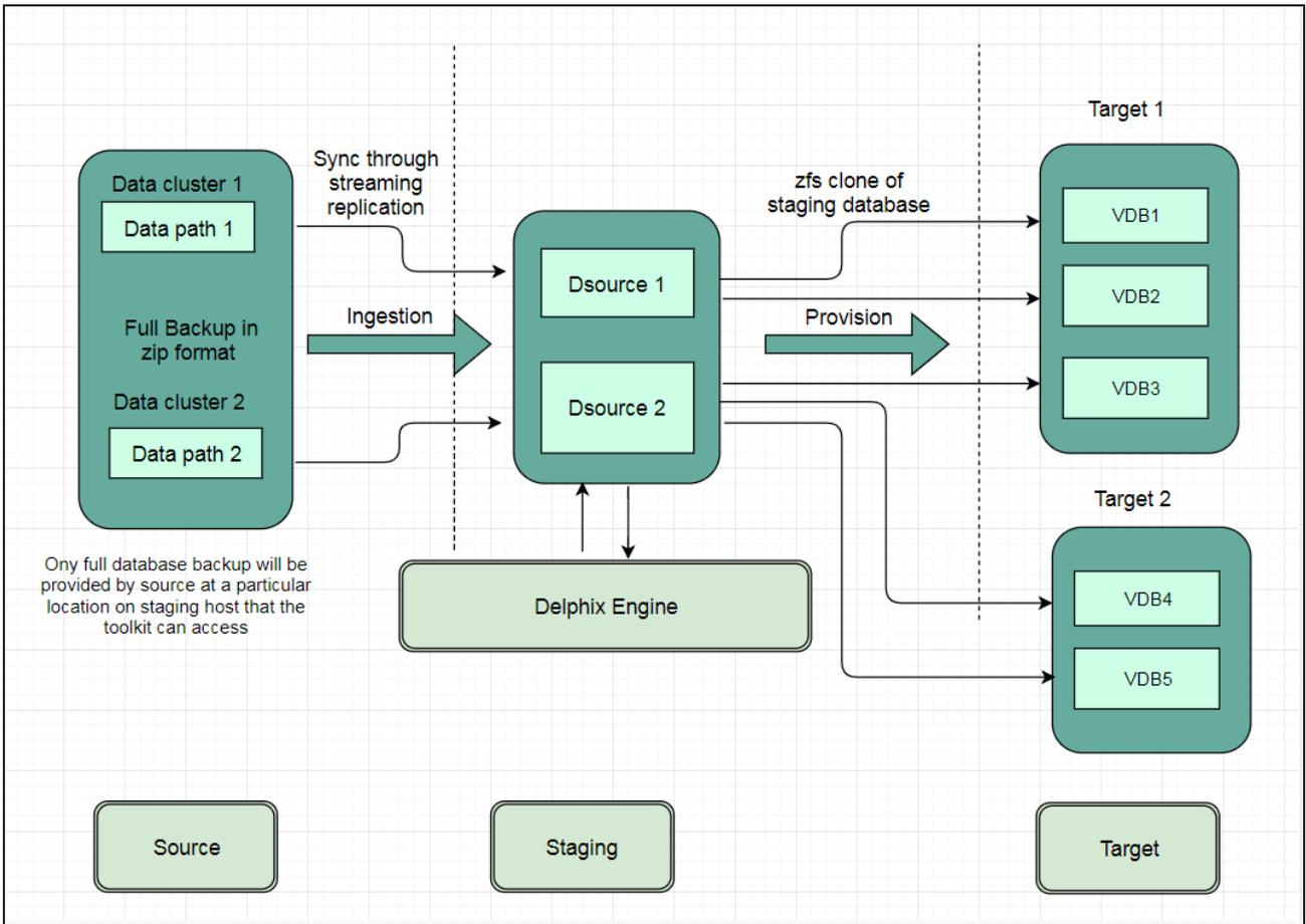
Delphix for PostgreSQL Architecture with Customer Initiated Backup Ingestion + WAL apply for resync between Source and dSource
