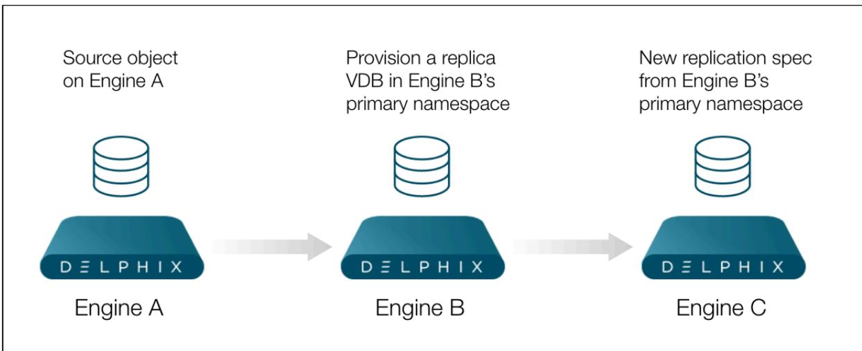
1. **Engine A Replicates to Engine B**
