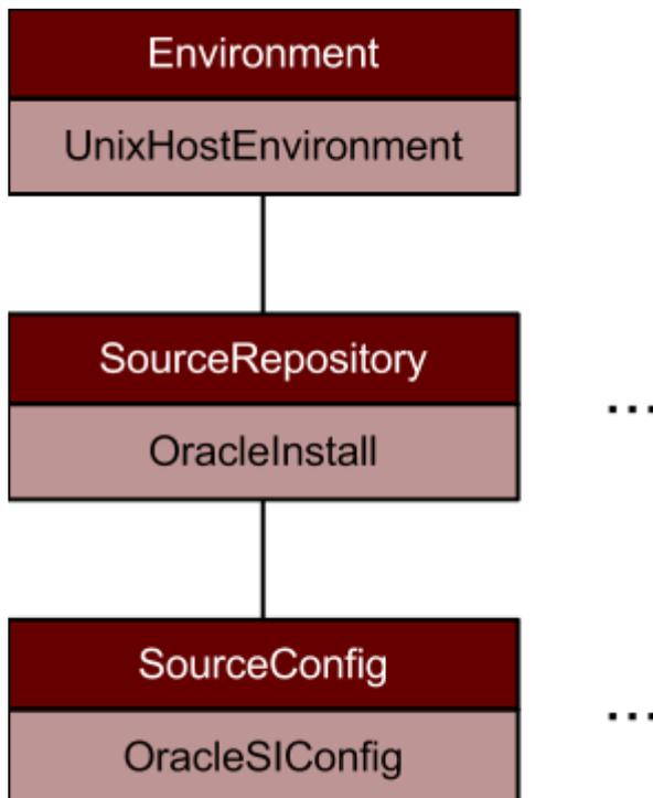
The generic type is listed in the top portion of each box, with an example of the Oracle single instance objects in the lower portion of each box. Each of these objects can contain multiple child objects with it.
