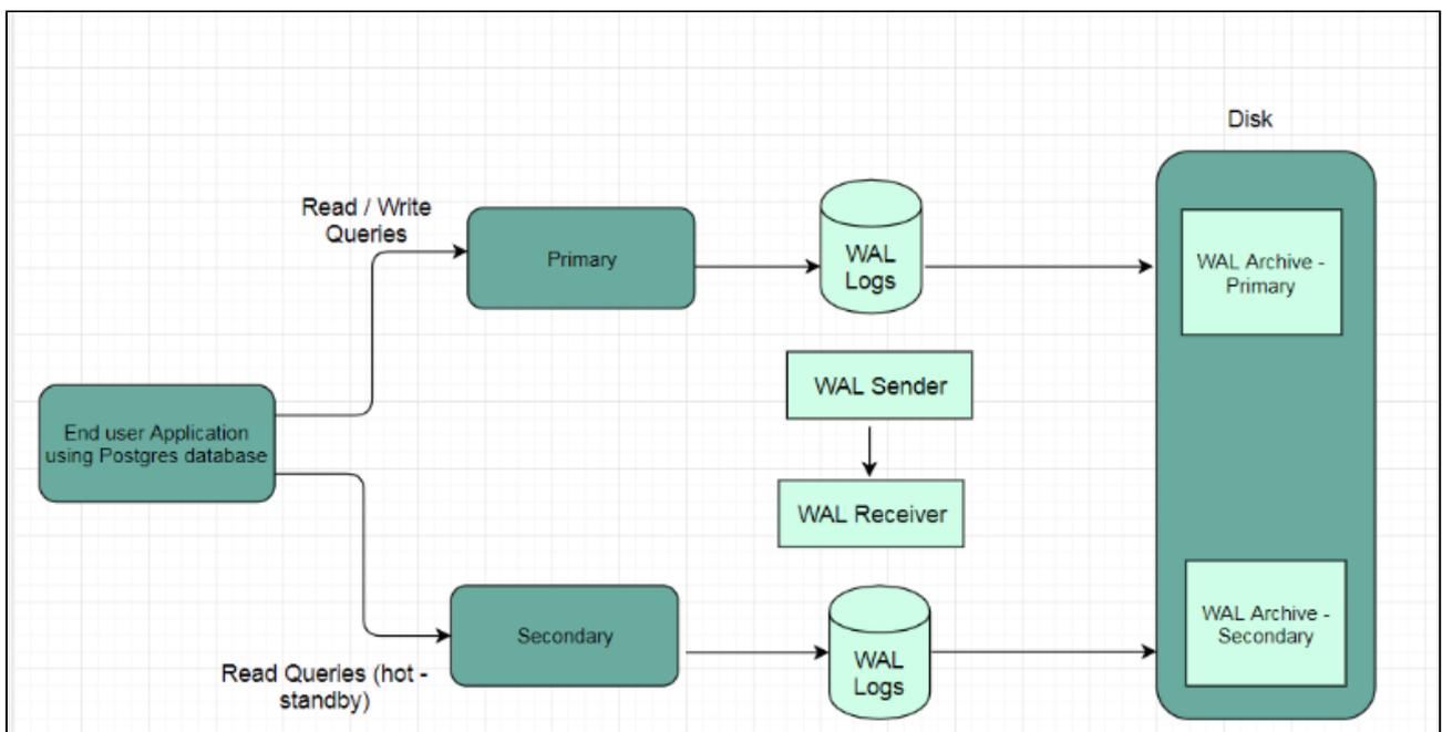
Delphix leverages this feature by capturing the replication stream via file-based log shipping or Streaming WAL records depending on your PostgreSQL configuration. Below is the same PostgreSQL replication architecture diagram with Delphix use case overlaid:
