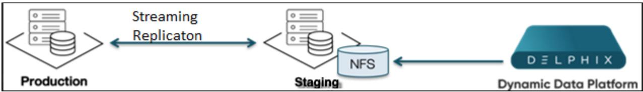
Delphix for PostgreSQL Architecture with Customer Initiated Backup Ingestion + PostgreSQL Streaming Replication between Source and dSource
