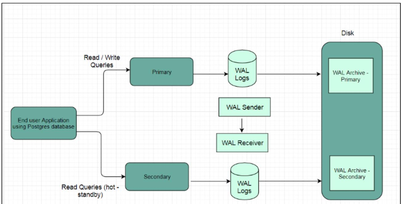
Delphix leverages this feature by capturing the replication stream via file-based log shipping or Streaming WAL records depending on your PostgreSQL configuration. Below is the same PostgreSQL replication architecture diagram with Delphix use case overlaid:
