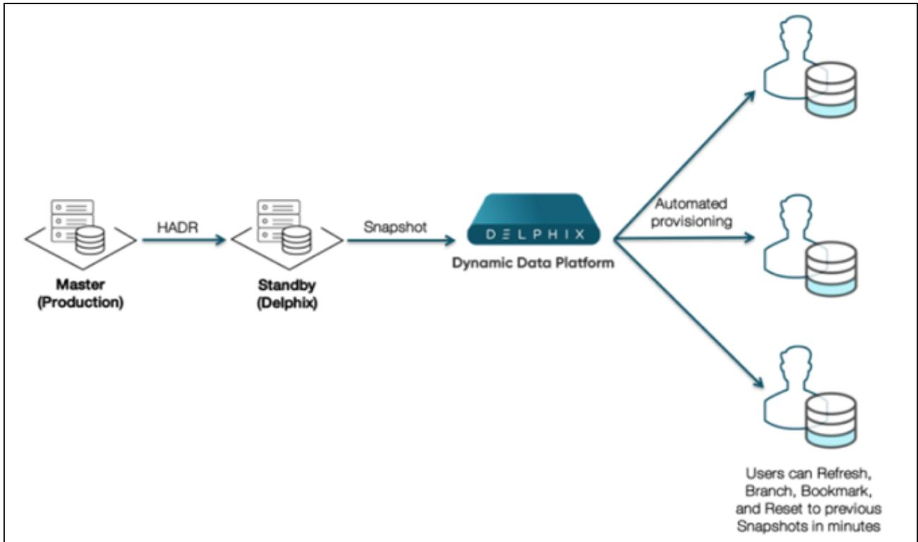
Delphix uses a Standby server called “Staging” to support the data ingestion process. There are multiple benefits of having a Staging server between the Db2 Source Instances and the Delphix Dynamic Data Platform:
