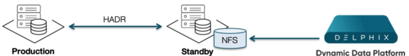
The linking process sets up a database inside an instance on the standby server and uses this as a HADR standby for the primary database. The staging instance must have access to a recent backup copy of the database that will be used to restore the initial copy of the dSource. Once the restoration process is complete, Delphix will issue the
