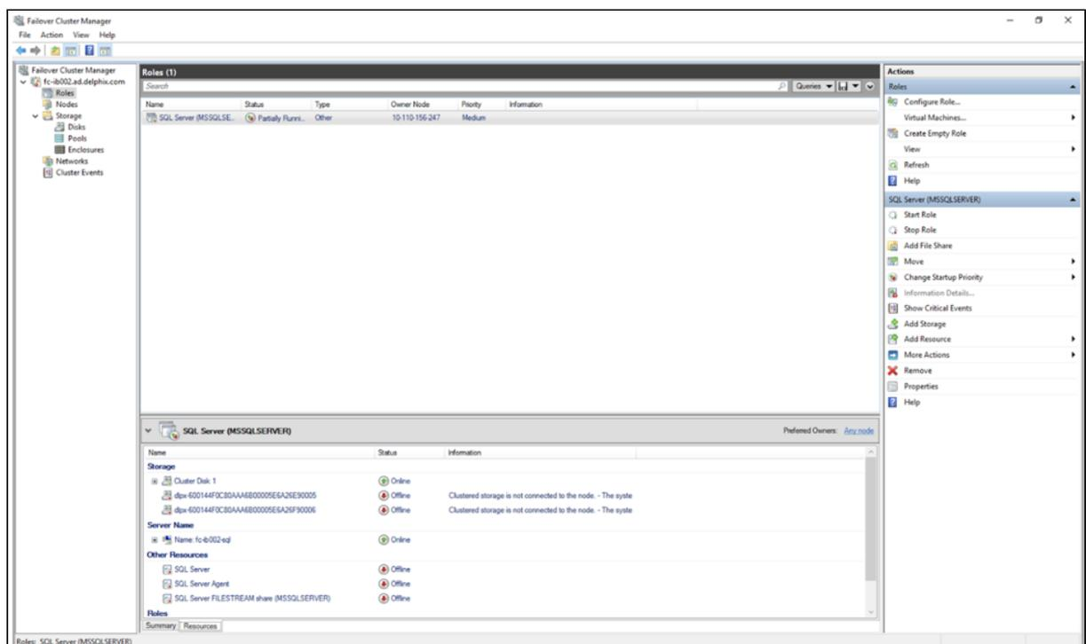
4. In order to fix the state go to the **Storage** section and select **Disks**. The **dlpx-XXXXXXXXXX** mounts attached to the Cluster Disk will be in offline states. These mounts will be equal to the total number of VDBs
