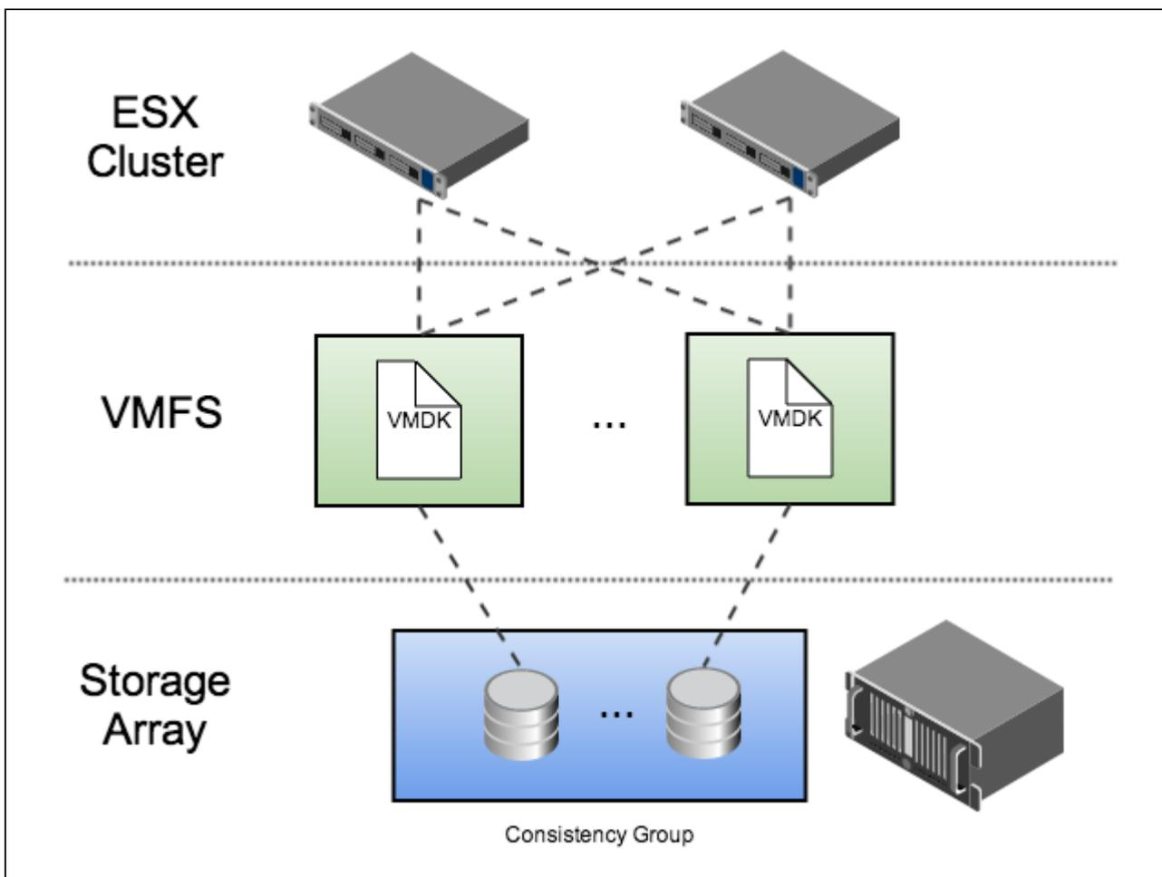
This architecture is designed to isolate I/O traffic to individual LUNs while using the most commonly deployed VMware components. In this example, each VMDK file is placed in a separate VMFS volume. Each volume is exported to every node in the ESX cluster, allowing the Delphix Engine to run on any physical host in the cluster.
