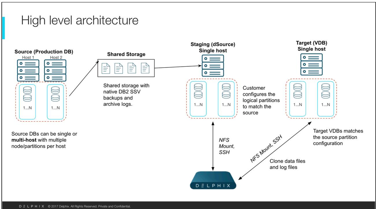
While using DPF, the DPF environment for Db2 staging and target should be configured on separate hosts. Also, staging and target should be configured with the same number of logical partitions as the number of partitions in the source node.
