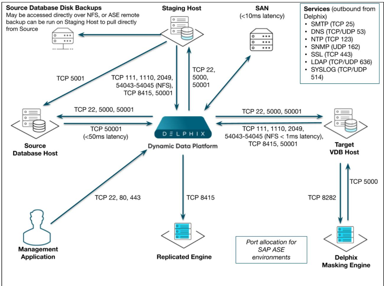
Refer to [Managing SAP ASE Environments](#) for information on SAP ASE environments. The Delphix Engine makes use of the following network ports for SAP ASE dSources and VDBs:
