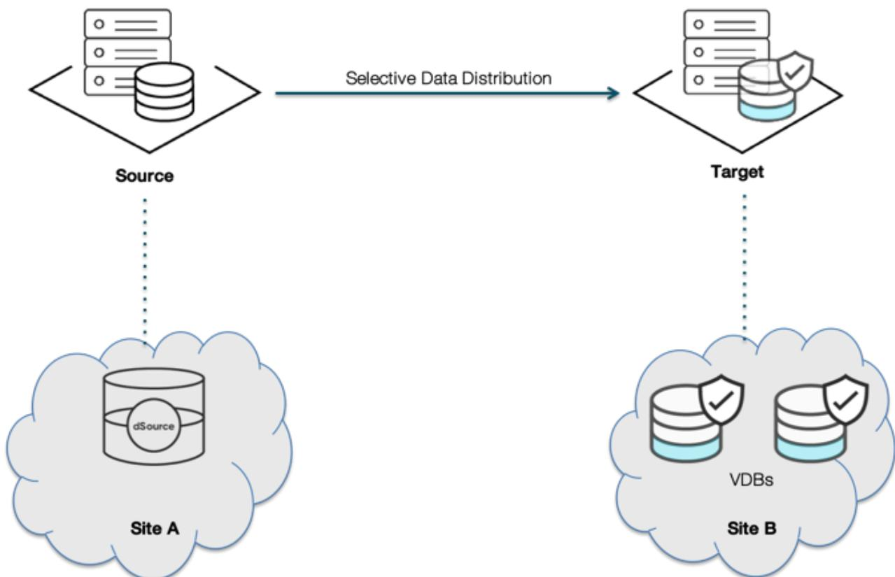
Because there is no failover, this technology can support more complex topologies such as 1-to-many and many-to-1. Chained distribution (replicating from Site A -> Site B -> Site C) is not supported.
