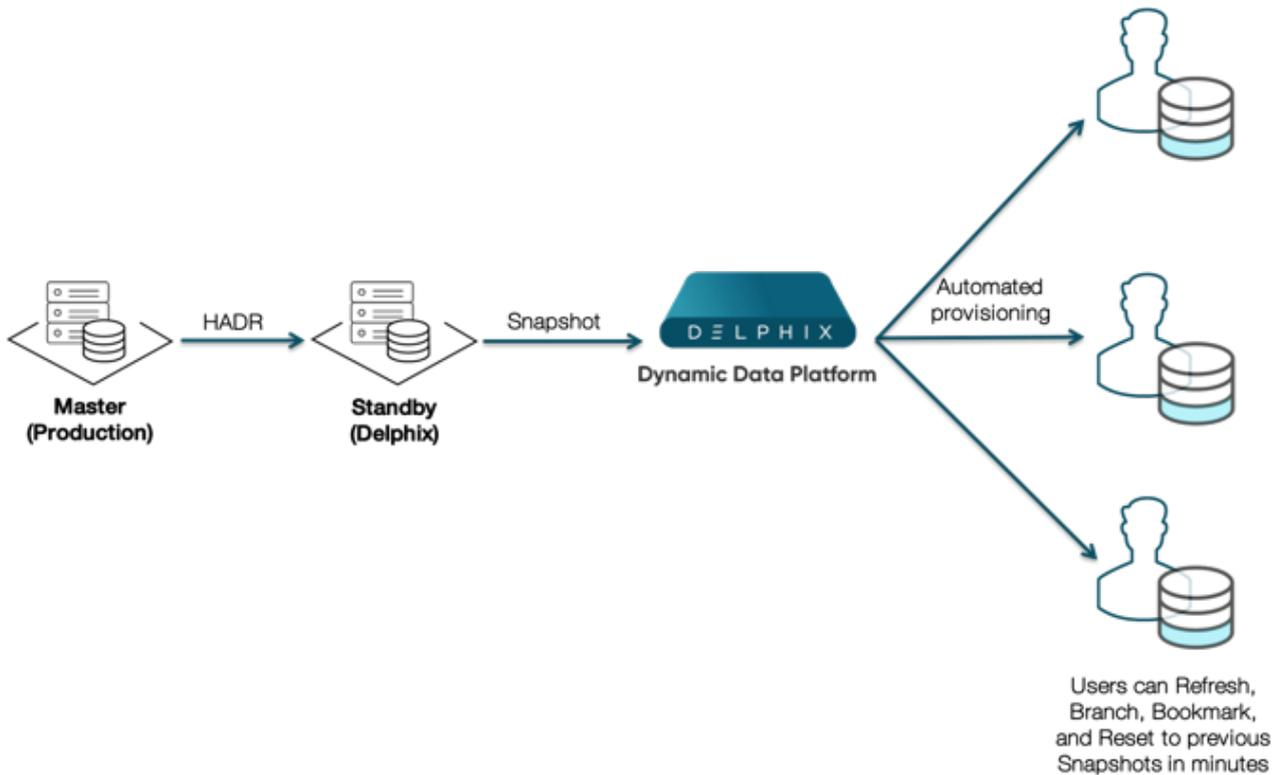
Delphix uses a Standby server model along with Db2s High Availability Disaster Recovery feature to ingest data and stay in sync with the source database. The standby server is then snapshotted by the Delphix Engine and the snapshots can be provisioned out to one or more target servers.
