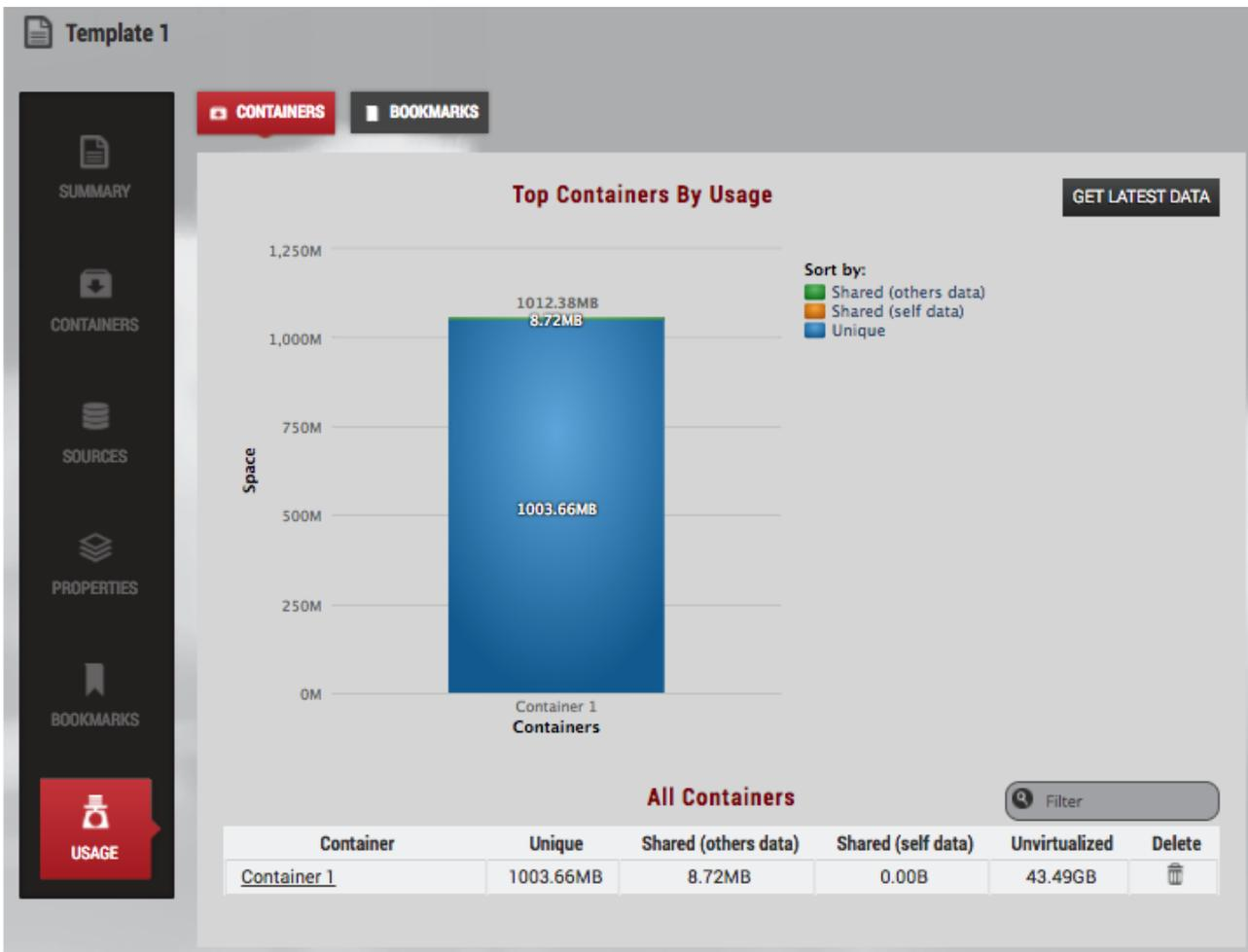
The stacked bar graph shows information about the top 10 space users. You can re-sort the graph based on the fields in the **Sort by** legend on the top right-hand corner of the screen as seen in the image above. For example, if you want to know which data containers are sharing the most data with others, you can un-select **Shared (others data)** and **Unique** by clicking them in the legend.
